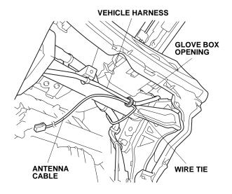
36. Route the antenna cable through the glove box opening and toward the center panel.
