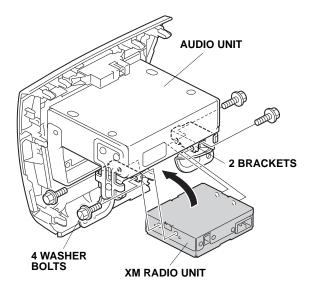
21. Tighten the two washer bolts installed in step 19.
