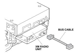
25. Plug the 2-port subharness into the audio unit connector and into the bus cable connector.
