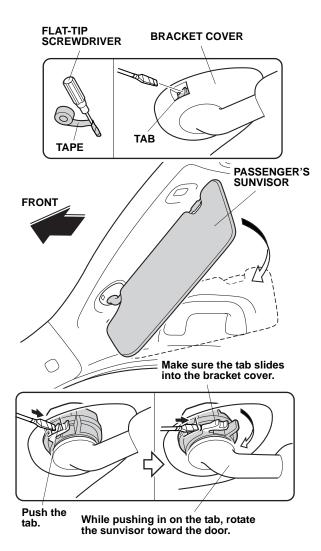
Unplug the vehicle connector, and remove the passenger's sunvisor.
