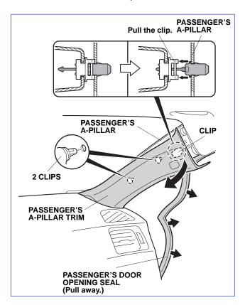
To prevent clips from falling into the body panel area, carefully insert a shop towel between the passenger's A-pillar and the passenger's A-pillar trim.
