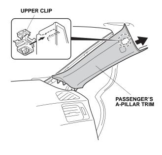
5. Remove the remaining upper clip from the passenger's A-pillar.
