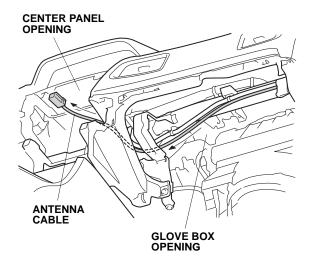
37. Route the antenna cable out the center panel opening, and align it with the other vehicle connector.
