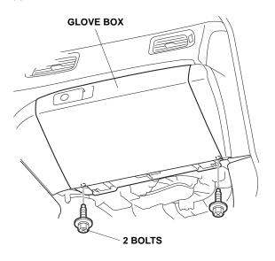
17. Remove the glove box (three self-tapping screws and unplug the vehicle connectors).
